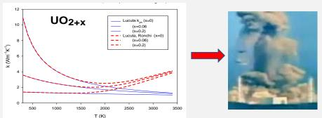
Therefore we investigate Enhanced Accident Tolerant Nuclear Fuels with enhanced thermal conductivity by electrons and high uranium density (no enrichment needed).
